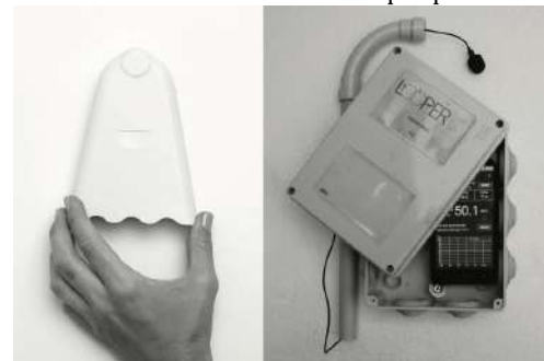
Fig.2 – low-cost sensors example: on the left the AirBeam to collect air quality data, on the right the Noise Box to collect data about noise levels. Credits: HabitatMap and luav.
