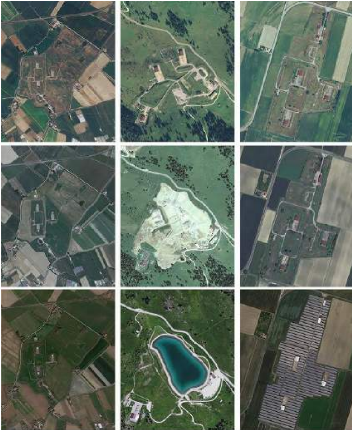
Figure 2. Orthophotos from 2006, 2012 and 2021 of three former Nike missile sites (Bovolone, Base Tuono and Zelo). The images show the similar initial layout, with three launch areas and logistic buildings, and the different evolution of the areas' uses: Bovolone is unused (except for a building at the entrance and the road used by a cyclist association); Base Tuono is now a museum and naturalistic area with an artificial lake; Zelo is a photovoltaic plant.
