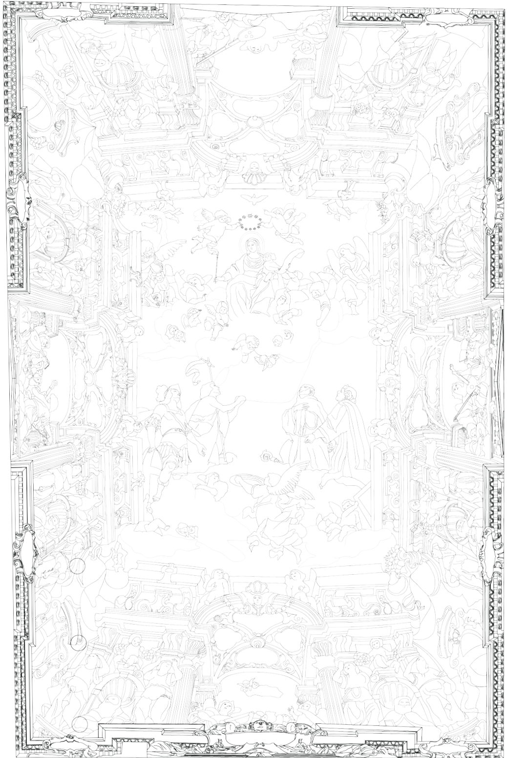
Fig. 4. Redrawing of the ceiling based on the orthophoto (elaboration by E. Adam and G. Massaro).
