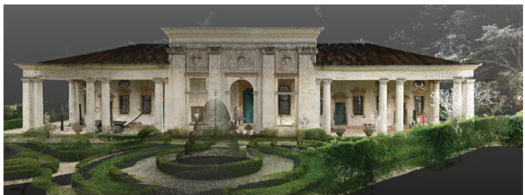
Fig. 3. Point cloud obtained through laser scanning, Villa Valmarana (graphic elaboration by the authors).
