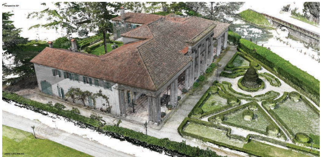
Fig. 2. Point cloud obtained from the photogrammetric survey, Villa Valmarana (graphic elaboration by the authors).
