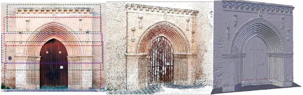
Fig.01 Photographic scanning, point cloud and mesh obtained.
