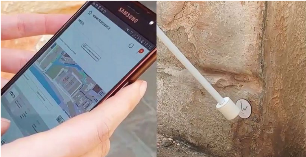
Fig.03 TAG installation, geolocalization and data integration via mobile App.
