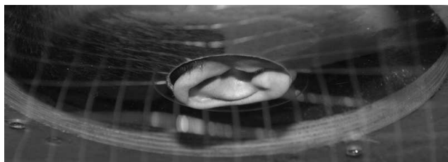
Figure 1: The pinna isolation device used for PRTF measurements.
