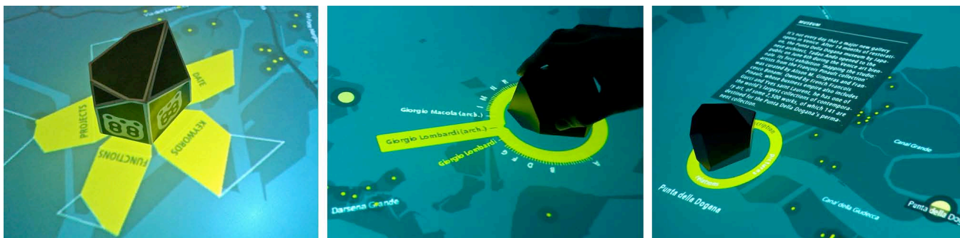
Figure 2. Interaction sequence with the tangible object, starting with a) selecting one of the facets, b) choosing a specific entry from the radial menu, and c) browsing through further metadata and media of a selected project.
