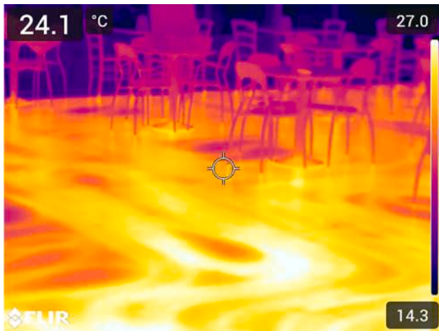
Fig. 16. RF on: piping emitting heat.
