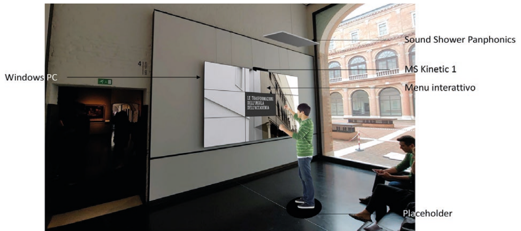
Fig. 2. Devices of the new interactive installation.
