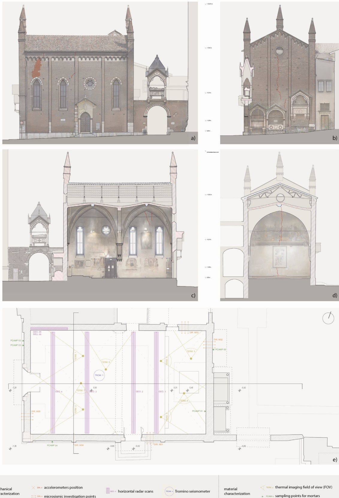
Fig. 1. Università Iuav di Venezia, 2024. Integrated Geometric Survey and Characterisation of the Crack Pattern. (a) South elevation showing the Crack SO and previous scuci-cuci repair areas; (b) East elevation showing the Crack EV; (c) Longitudinal section of the church; (d) Transversal section; (e) Ground-floor plan with the location of the diagnostic investigations, including ambient vibration testing, microseismic measurements and thermographic surveys.
