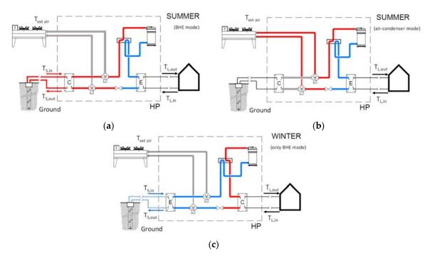
**Figure 4.** Scheme of the new hybrid heat pump: (a) operation in cooling mode using borehole heat exchangers; (b) operation in cooling mode using air-condenser; (c) operation in heating mode using borehole heat exchangers.
