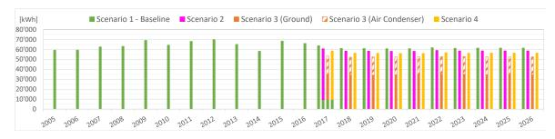
Figure 10. Annual electrical consumption of the heat pump for each simulated scenario.
