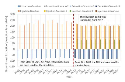
Figure 7. Ground heat extraction-injection rate in each simulated scenario.
