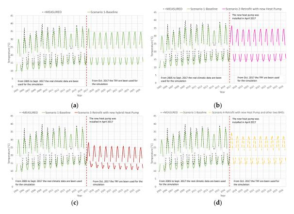
**Figure 6.** Mean monthly outlet fluid temperature from the borehole heat exchangers: measured values from 2006 to 2017; simulated values in (a) *Scenario 1*, (b) *Scenario 2*, (c) *Scenario 3*, (d) *Scenario 4*.
