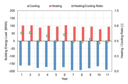
**Figure 5.** Calculated annual thermal load of the building from 2005 to 2016 and heating to cooling energy demand ratio.
