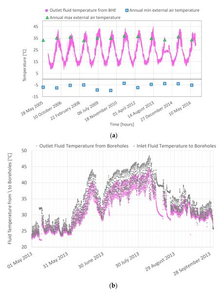
**Figure 3.** Measured hourly fluid temperature: (a) outlet fluid temperature from borehole heat exchangers with annual minimum and maximum external air temperatures, (b) inlet and outlet fluid temperature to/from borehole heat exchangers from May to September 2013.
