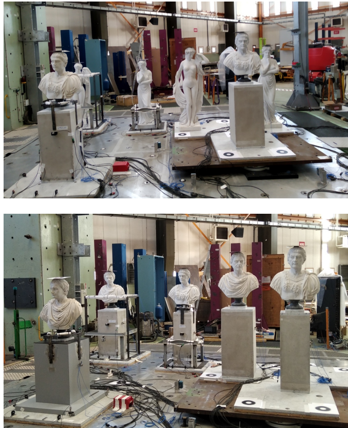
Figure 4. Two different testing configurations considered. The busts on the right-hand side of the photo are placed on friction pendulum isolators.
