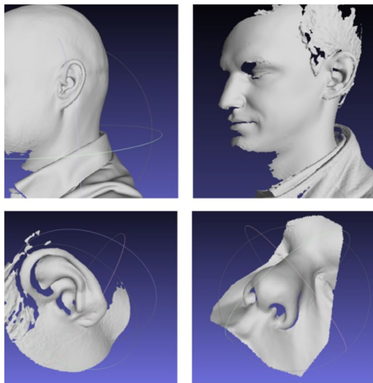
Fig. 4 Examples of facial scans using handheld scanners (Go!SCAN, top row; SIMSCAN 3D, bottom row) for post-processing in MeshLab
