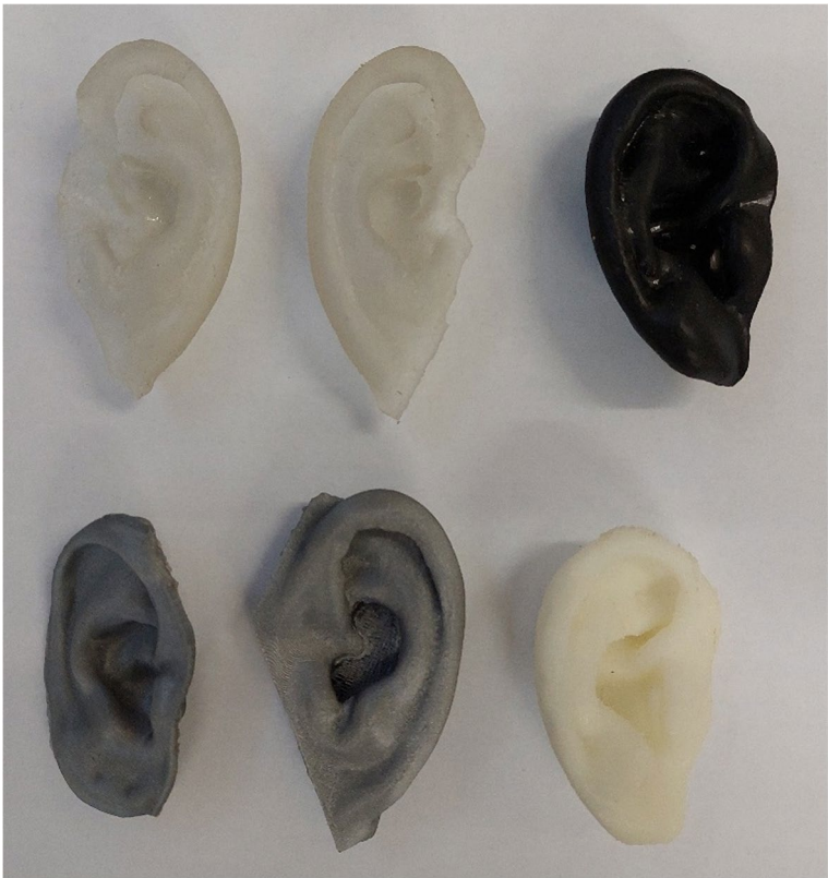
Fig. 10 Examples of printed replicas using hard polymer and synthetic resin. The top left is the mirrored version of the top middle replica
