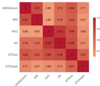
Figure 16. Linear correlation between selected omnidirectional roughness indices. STDslope: standard deviation of slope; SA: area-based method; STDres: standard deviation of residual surface, with trend computed with a local polynomial of order 1; NVD: normal vector dispersion; RRI: radial roughness index; MADk2omni: omnidirectional MAD with DDs of order 2 and a lag of 1 pixel.
