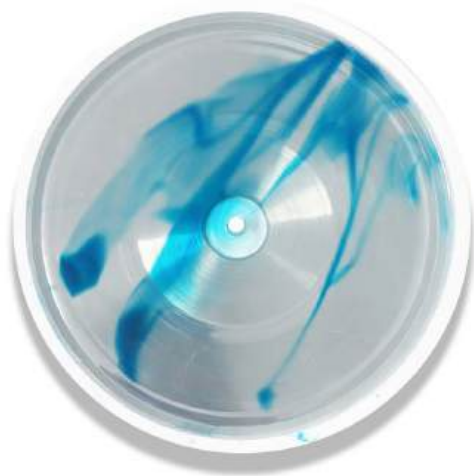
Fig. 5. A bio-based phonographic disc composed of 97.5% water and natural gelling agents, compatible with traditional production techniques and offering acoustic performance equivalent to that of vinyl.
