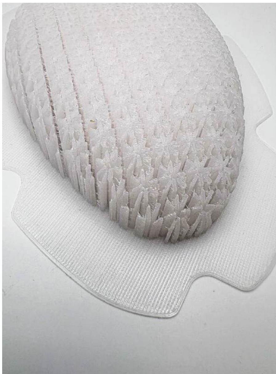
Fig. 3. Morphological Protection. Prototype of an adaptive protection system for motorcyclists. Compared to traditional systems, it uses less material while providing the same level of performance.
