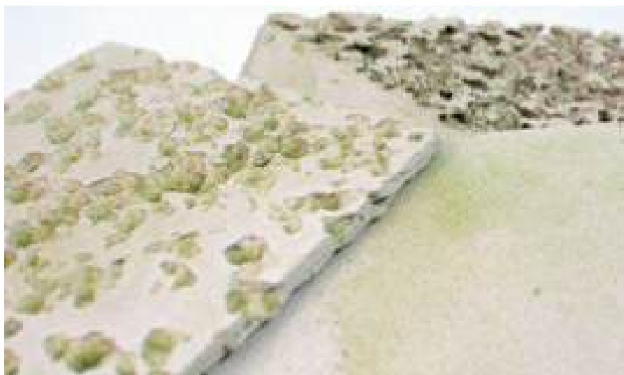
Fig. 1. Continuities & Discontinuities – Samples of bioreceptive ceramics with multiscale porosity obtained from pyrolyzable organic waste, undergoing colonization by a cyanobacterial biofilm.
