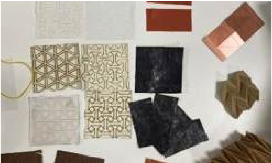
Fig. 4. Auxetic Behavior and Design – Samples of standard materials transformed using auxetic geometries: structures with a negative Poisson's ratio that change their mechanical behavior under stress.
