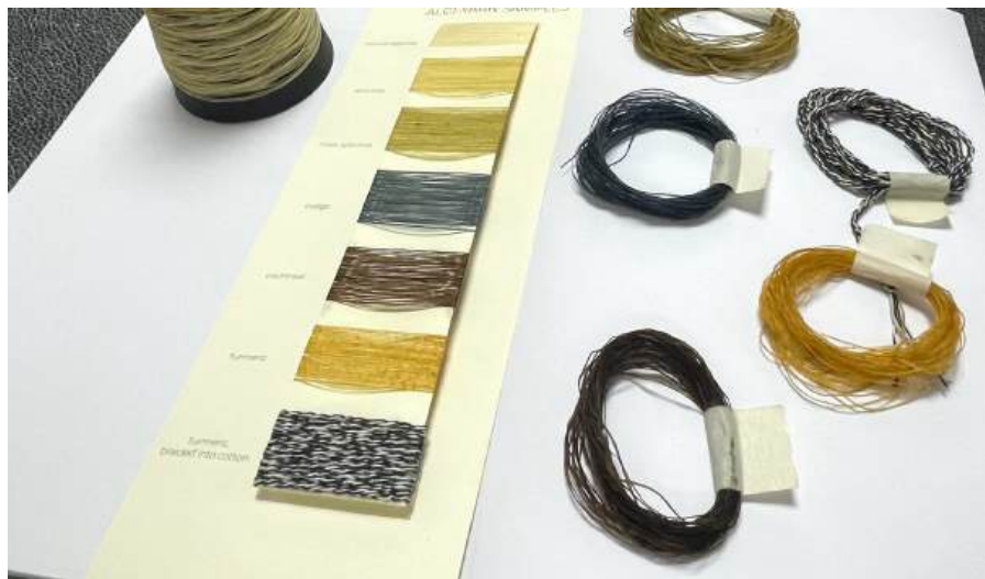
Fig. 8. Algi-Yarn – Continuous yarns made from sodium alginate, produced using an open-source desktop spinning machine through mechanical adaptations and iterative reformulations of the material.
