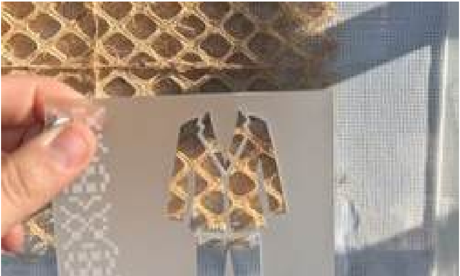
Fig. 3. Weaving the Future – Lattice structures created by guiding the root growth of grasses through PLA molds inspired by crochet lace patterns.
