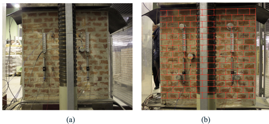
Figure 4. (a) Masonry panel under compression (b) Grid superimposed over the existing masonry texture (c) Grid as a guide to define the rigid blocks
