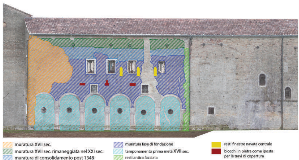
Fig. 5. Identification of the different wall portions and surviving elements in the northern wall of the monastery (elaboration by authors).
