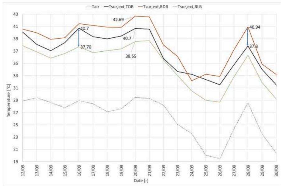
Fig. 11. Maximum temperature on external surfaces of the specimens during the monitoring period.
