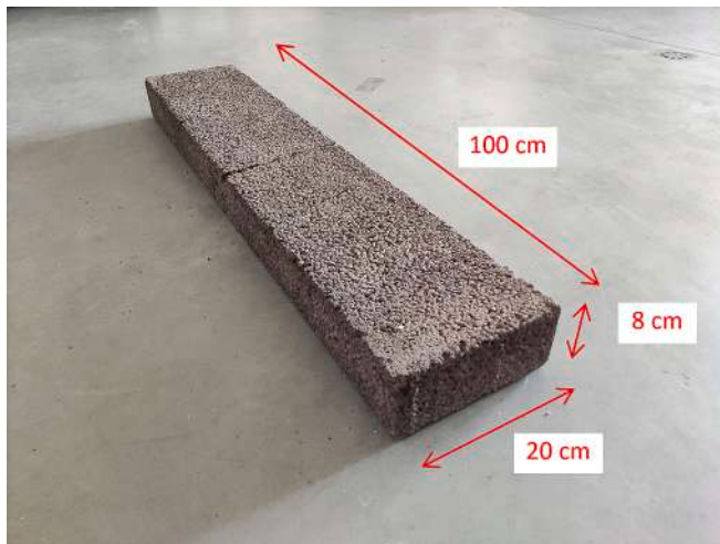
Fig. 1. Example of Recycle® porous block (dark version).
