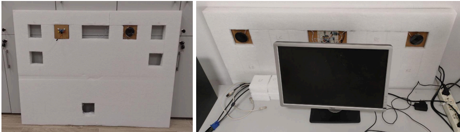
Figure 5: The panel used for the prototype for the first solution. On the left it's shown in full view with the housings for the electronic components and two example cardboard "modules". On the right, it's shown housed behind a desk where the functionalities of the various sensors were evaluated. During the tests, the facade was then covered with fabric to test the sensors' response in this condition.
