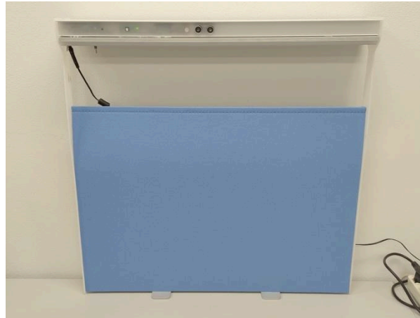
Figure 6: Prototype with sensors inserted into the ALL-LED extruded profile, with the addition of a LED strip for lighting.
