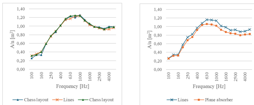
Figure 1 (left): Equivalent absorption area per panel A/n of elements under test with different arrangement modes (checkerboard layout and thinned lines) for 53.3% reverberation chamber occupancy compared to the maximum occupancy made.
