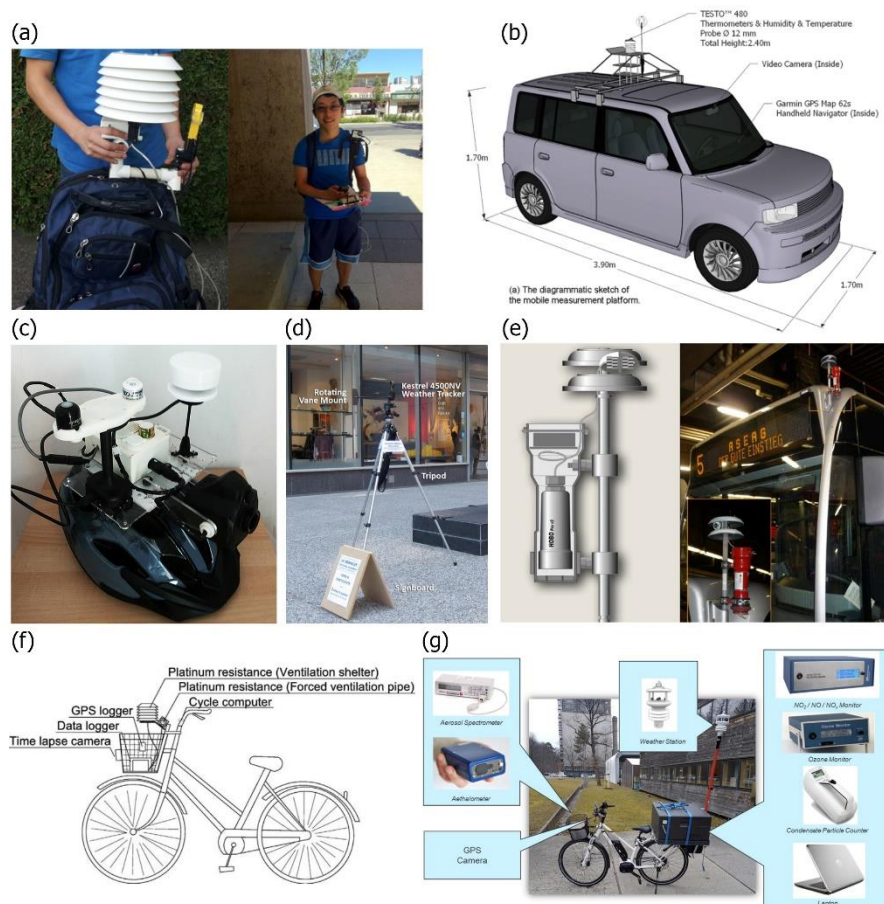
Figure 33. Examples of mobile traverse systems that have been used in previous studies. (a) A mobile monitoring setup composed of a radiation shield containing a temperature sensor, a portable weather station and a video camera (Tsin et al., 2016); (b) A light-colored vehicle equipped with several sensors, a Global Positioning System (GPS) and a video camera (Shi et al., 2018); (c) A wearable monitoring system with several embedded sensors as well as a camera and a GPS (Pigliatile and Pisello, 2018); (d) A semi-stationary weather station composed of a portable weather station, rotating vane mount, tripod, and signboard (Kim and Macdonald, 2016); (e) A local transport bus in Aachen, Germany, equipped with a self-built measurement device consisting of a temperature sensor and a GPS (Buttstädt et al., 2011); (f) A bicycle equipped with a temperature sensor and a GPS (Yokoyama et al., 2018); (g) A bicycle equipped with different sensors of air pollutants (Samad and Vogt, 2020).
