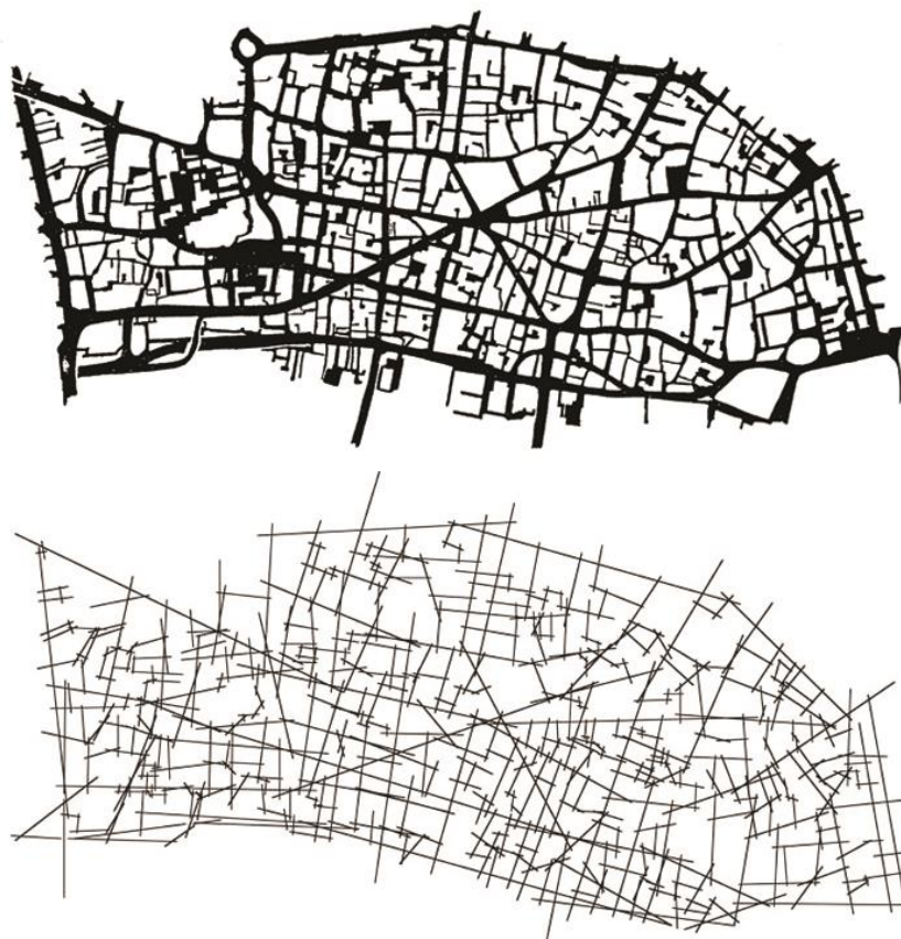
Figure 13. Figure-ground (top) and axial map representation (bottom) of the city of London. Reproduced from (Hillier, 1996, p. 117).
