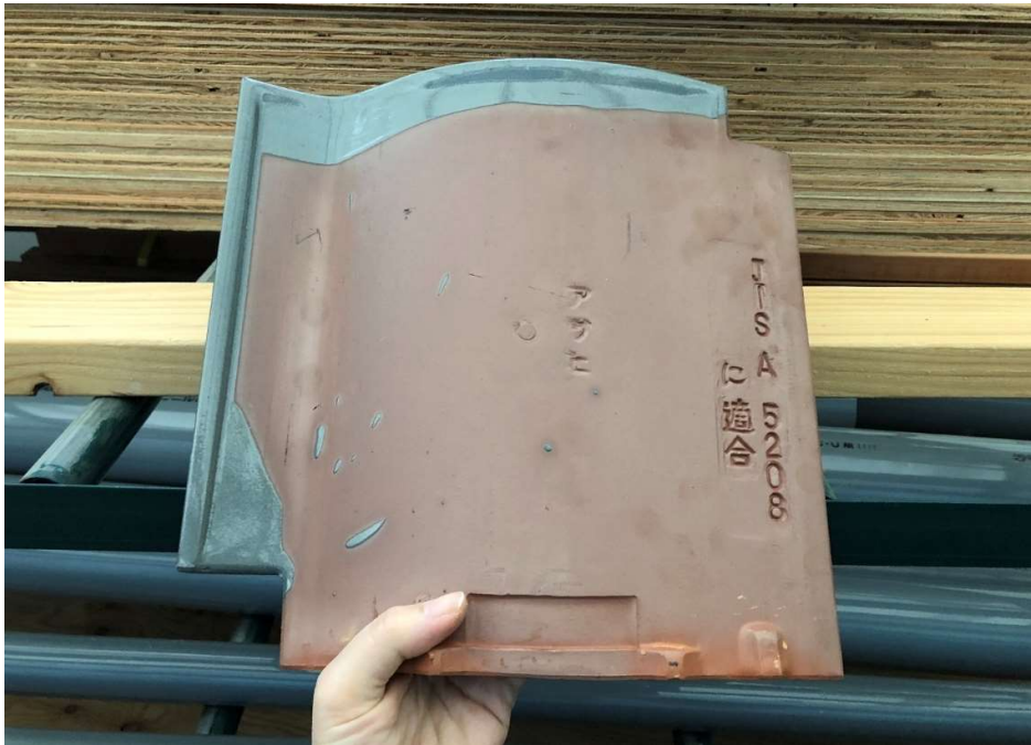
Figure 21 - Typical Japanese roof tile used to test wind-borne debris impact resistance of the building envelope at DPRI, Kyoto University.
