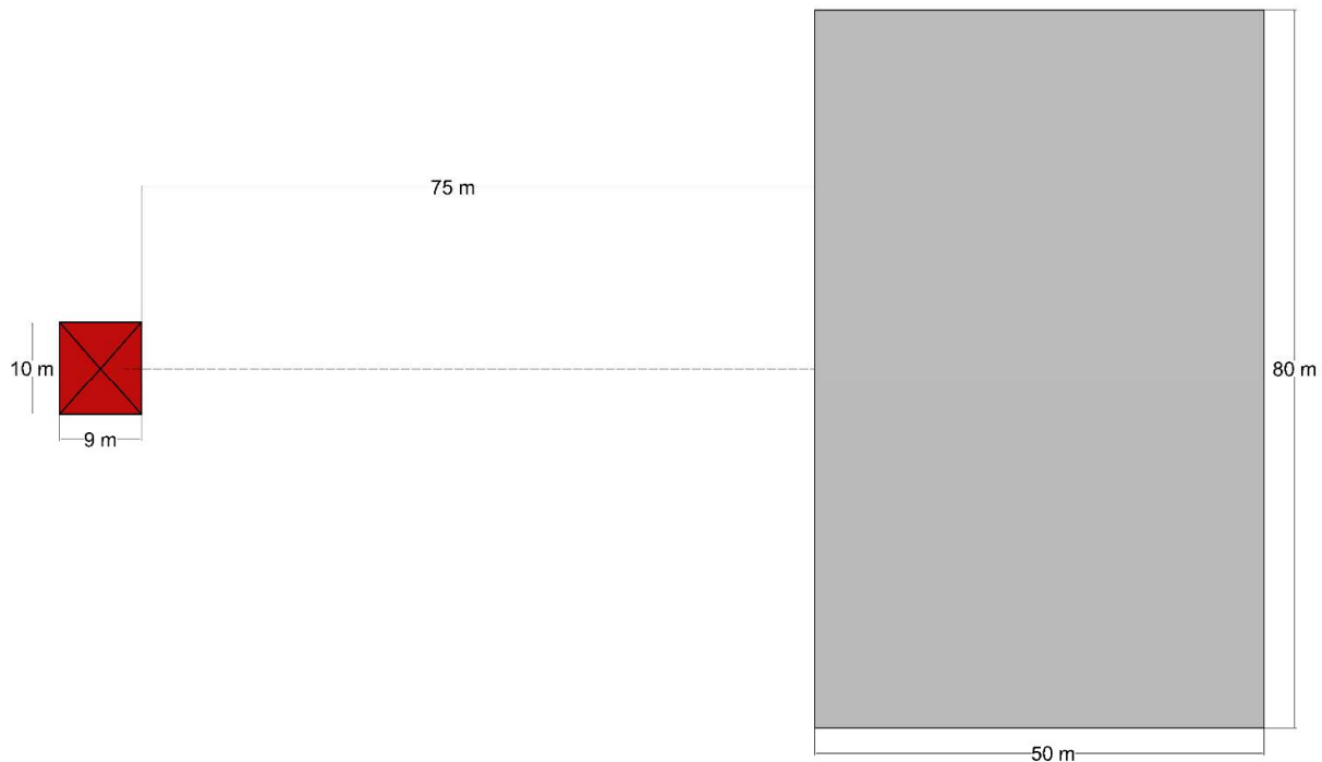
Figure 36 - Plan of the “source building” (red), “target façade” (grey) that is to be designed. Mean roof height is 10 m and one roof tile trajectory is reported with the dashed line.
