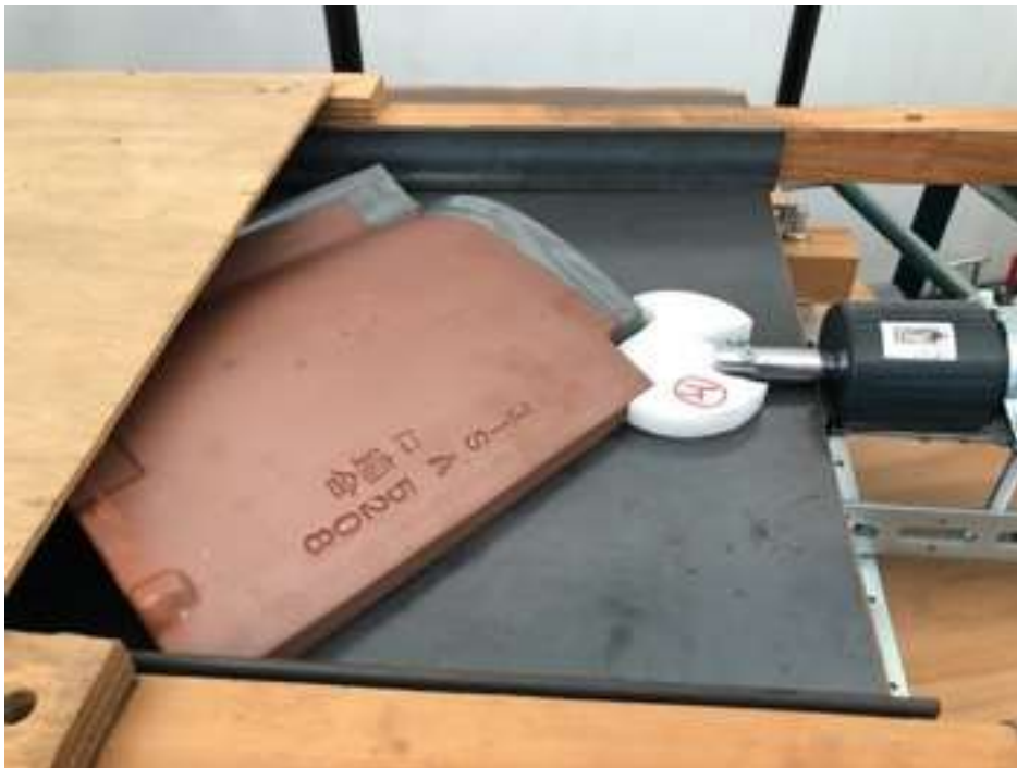
Figure 22 - Typical Japanese roof tile and air cannon adaptor equipment to shoot the tile through a glass sheet, DPRI, Kyoto University.
