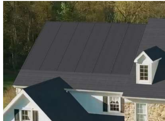
Figure 10: BIPV system installation rendering
