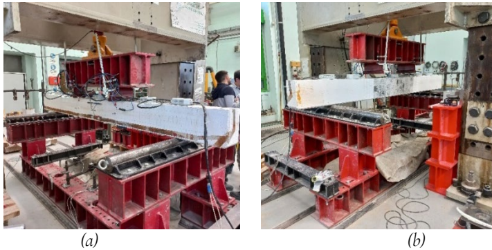
Fig. 3.12 Setup used in the second experimental series (a) Side with LVDTs; (b) Side with speckle pattern
