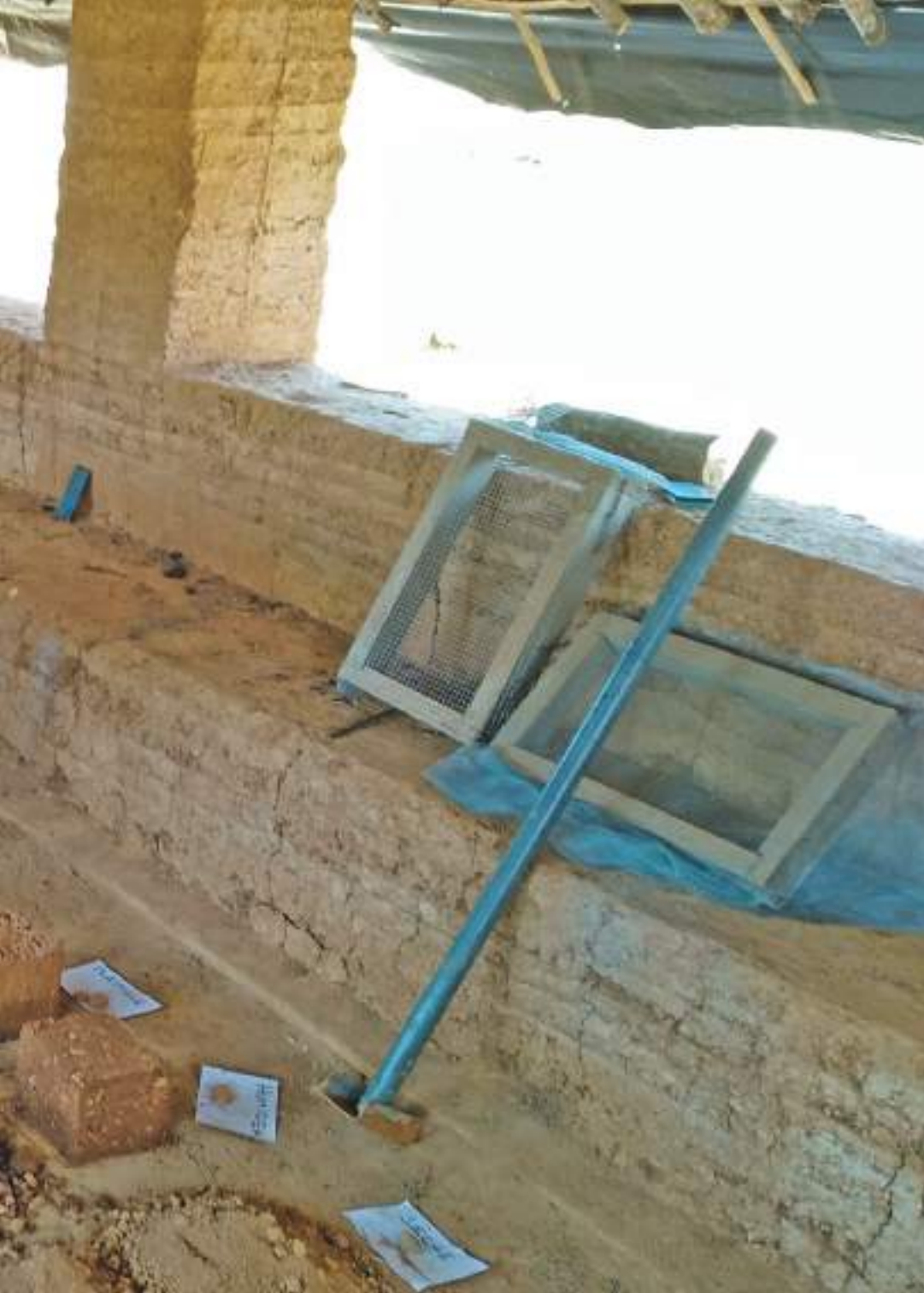
Côte d'Ivoire, Prikro, preparation of raw earth samples with different mixtures for the construction of the rammed earth components.
