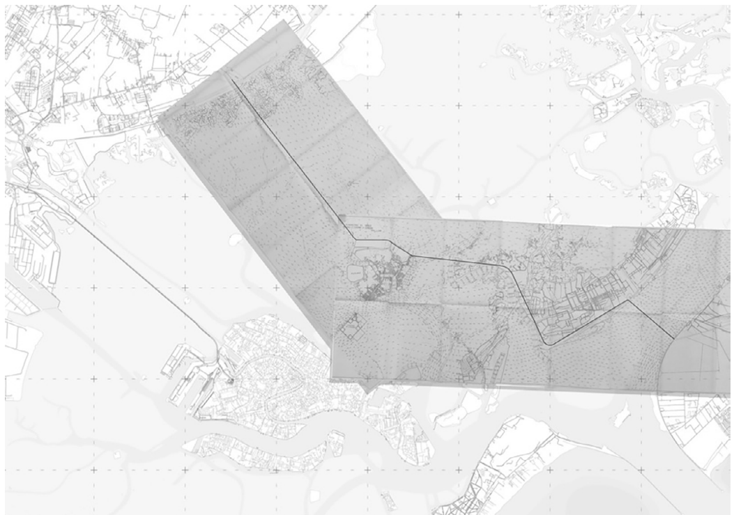
Fig. 3. Bathymetric points on georeferenced CTR with project overlay. Elaboration by G. Casarano.
