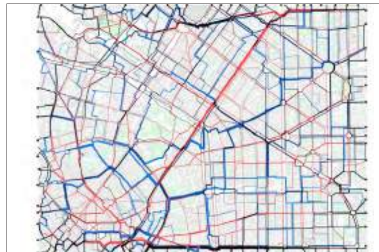
Fig. 1. Pedestrian flow diagram of shortest paths (in red) and coolest paths built on the average PET value (in blue). In black are highlighted the portions of routes where the two Pedestrian flow diagrams overlap.
