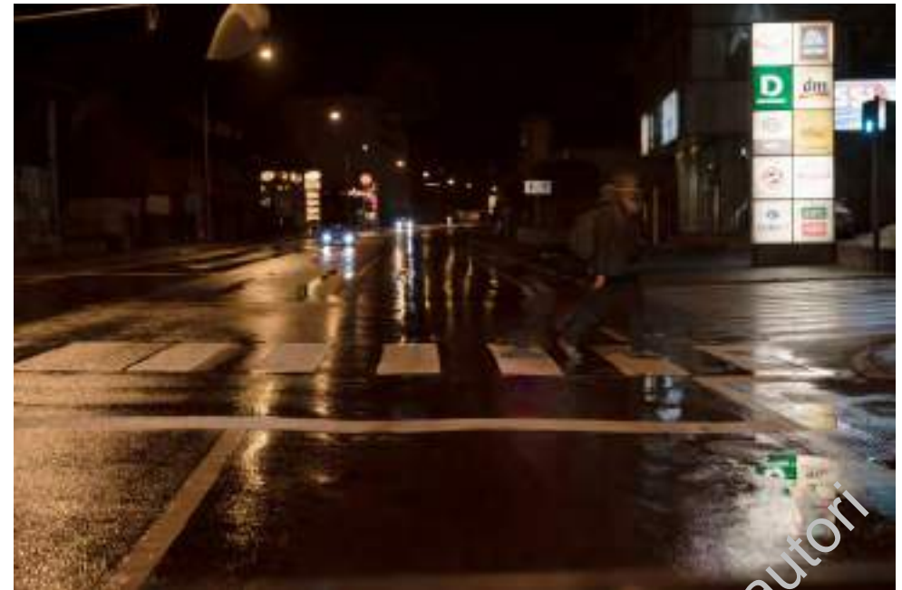
Fig. 1. The image highlights the poor visibility of the pedestrian walking along the pedestrian crossing due to low levels of contrast in public lighting (photograph © Siegrun Appelt).
