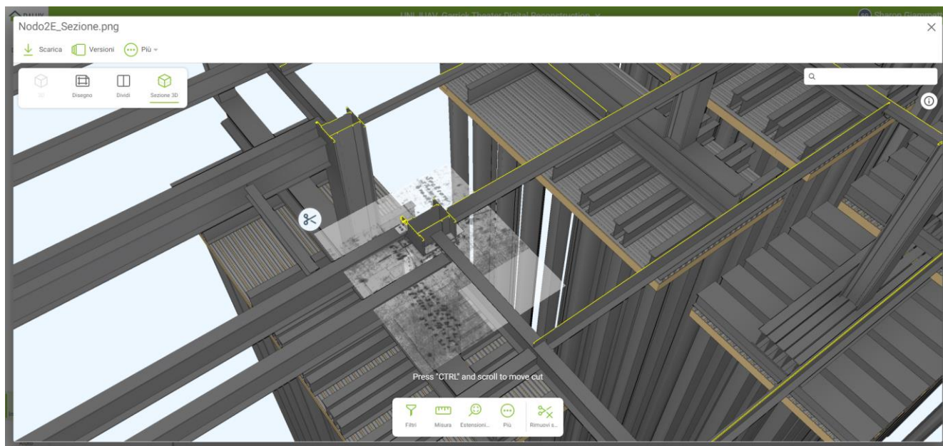
Fig. 14: Integration of historical 2D detailed documentation with IFC model in a CDE platform, to enrich and adding value to BIM model.
