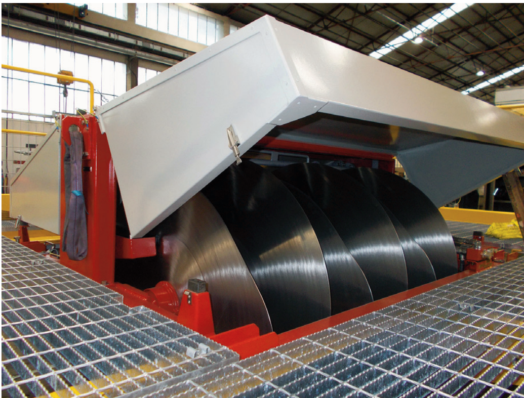
Fig. 2 | The disc structure of the current Discoil oil separator (credit: E. Marchetto, 2018).
