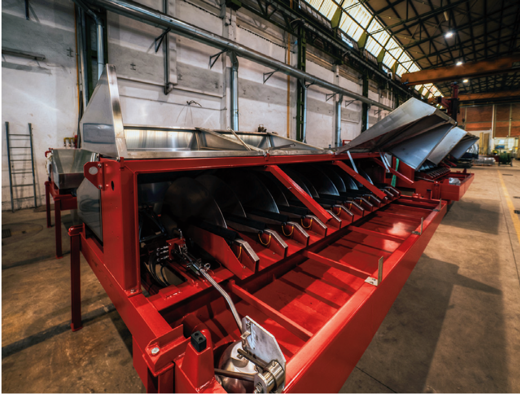
Fig. 1 | The Discoil in its current L10 configuration (with ten blades), manufactured at OCS (credit: M. Battaglia, 2024).
