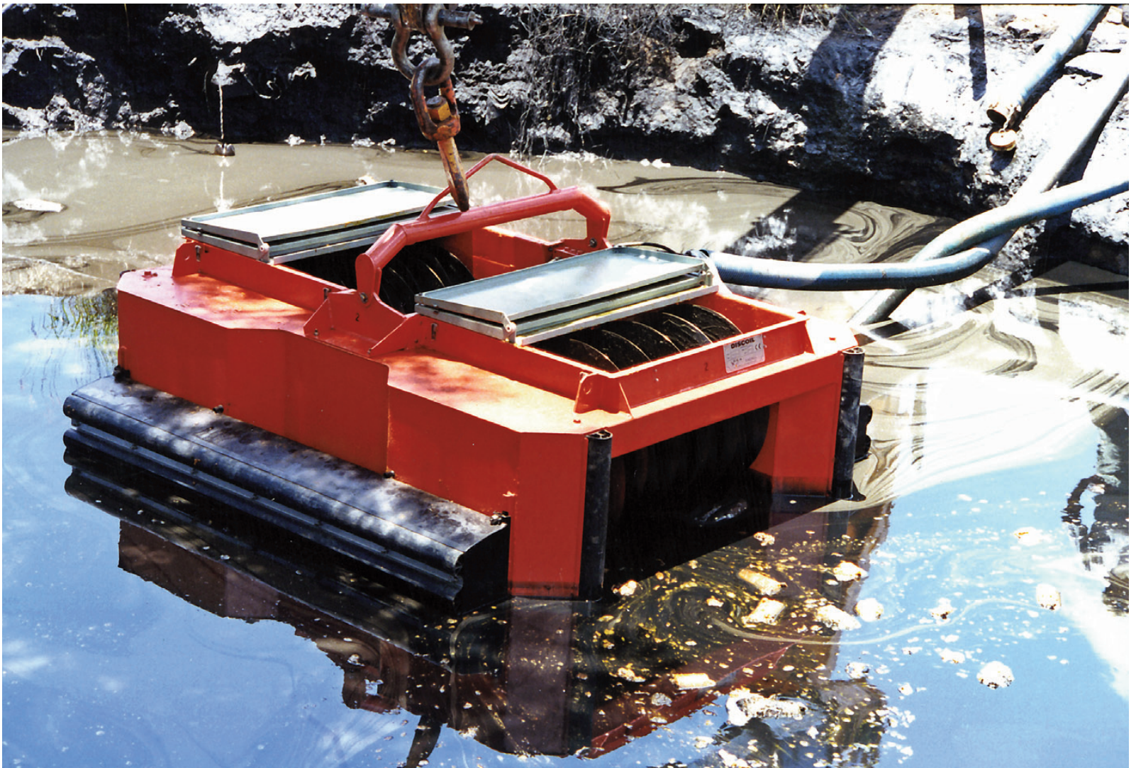
Fig. 7 | The Floating Discoil system in action in a lake (credit: OCS, 2008).
