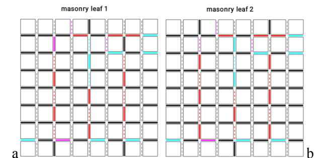
Fig. 7: Crack patterns for the leaves of the two-leaf masonry panel (failure types: cyan = tensile, red = shear, magenta = bending)
