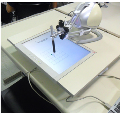
Figure 38 Prototype of robotic system for assisted hand-writing exercises based on Haptic 3D touch controller Novint Falcon
