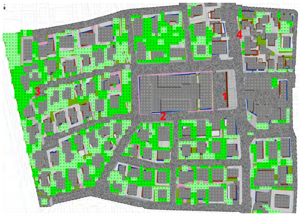
Fig. 5.3.4 The model area in ENVI-met used for the simulations of the “Asls”, “Cool pavements” and “Cool roofs” scenarios. The red numbers identify four characteristic points for which air temperature at 2 m above ground has been considered in the study
