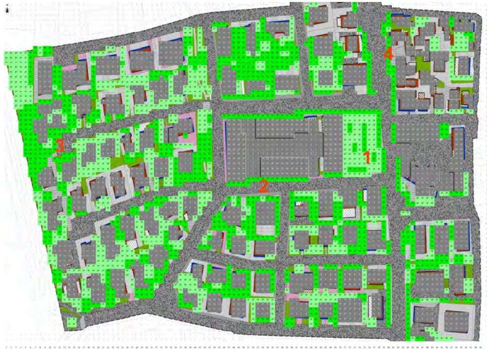
Fig. 5.3.5 The model area in ENVI-met used for the simulations of the “Green ground” and “Green ground + Cool pavements” scenarios. The red numbers identify four characteristic points for which air temperature at 2 m above ground has been considered in the study
