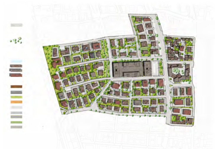
Fig. 5.3.5.13 Intervention 4 + summary of intervention 4. Albedo on private paved surfaces. Modify the reflectance on private surfaces
