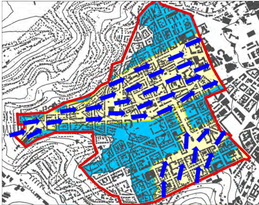
Fig. 5.5.16 Major cold air streams in Stuttgart-West. The yellow shaded areas mark areas with restriction to buildings to reduce the obstruction of existing streams.
