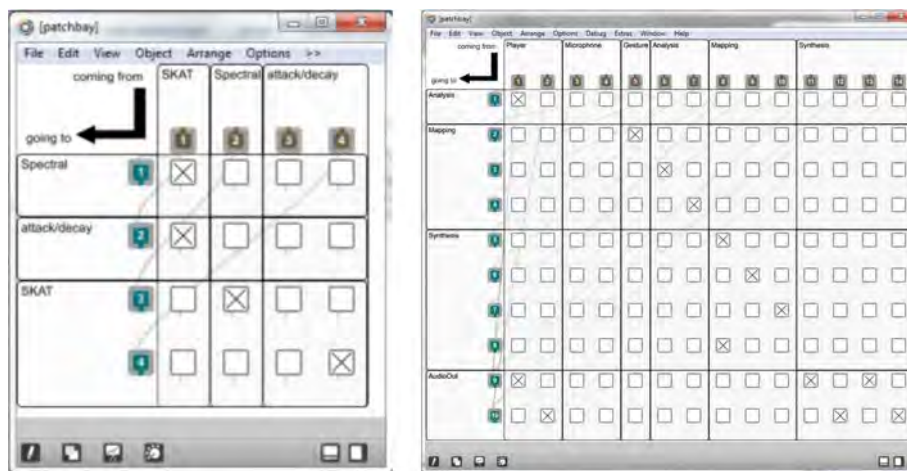
Figure 3. On the left, example of a patchbay for the analysis group. On the right, the global SkAT-Studio patchbay.
