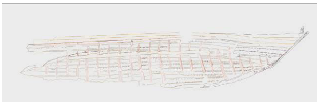
Figure 15. 3D vectorial model of the entire hull.
