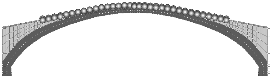
Fig. 5 Bridge with non-structural masses representing stone parapets.
