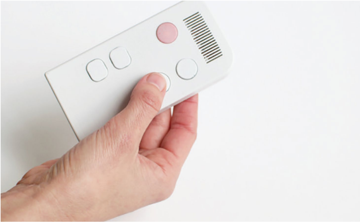
Figure 8. Product series: air conditioner remote controller. Supporting adjustment of temperature (musical diatonic scale), wind mode (frequency gate sound filter), and on-off modes (pitch shifting).
