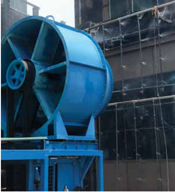
Figure 6.3. A façade assembly is tested for water-tightness under dynamic pressure façade testing at the Hong Kong Curtain Wall Testing Center. © Angela Mejorin
