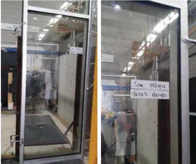
Figure 5.10. IMOC Windborne Debris Testing Procedure. A 4-kg timber missile is fired 40 m/s at a glass panel. Glass panel makeup: 6-mm HS + 6.08-mm PVB + 6-mm HS + 12 mm air + 6-mm HS. © JML-Craft
