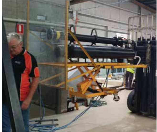
Figure 5.11. IMOC Windborne Debris Testing Procedure. While missiles were fired at the center of the glass, on the last test for SY-6168 IMOC, Port Hedland, the timber missile was fired at the corner at 40 m/s for comprehensiveness. Because of the equipment limitations, the missile had to be fired at the top corners. A forklift was used to achieve the required altitude. © JML-Craft
