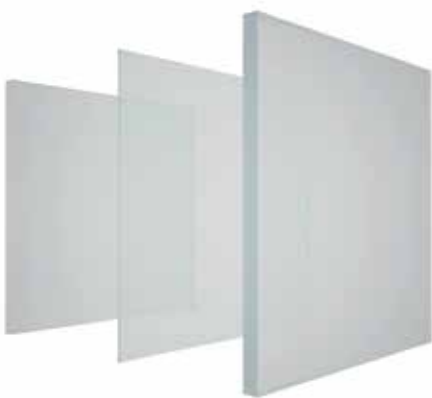
Figure 4.1. Laminated glass: two glass lites and one interlayer. © Michele Bettineschi
