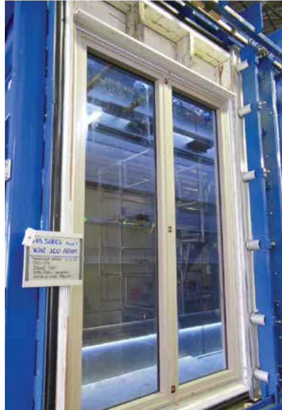
Figure 5.18. Australian Institute of Tropical Health and Medicine, fixed glazing performance mock-up test. © G. James Glass & Aluminium
