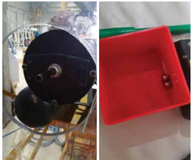
Figure 5.9. IMOC Windborne Debris Testing Procedure. The nozzle is then fitted with a steel ball bearing adapter. The steel ball bearing can be fired at the same specimen of glass if it passed the timber missile test. Five steel ball bearings are fired in five different locations. In general, the effect of the ball bearing on laminated glass is minimal. From discussion with the testing facility, the ball bearing has the greatest effect on monolithic glass. © JML-Craft
