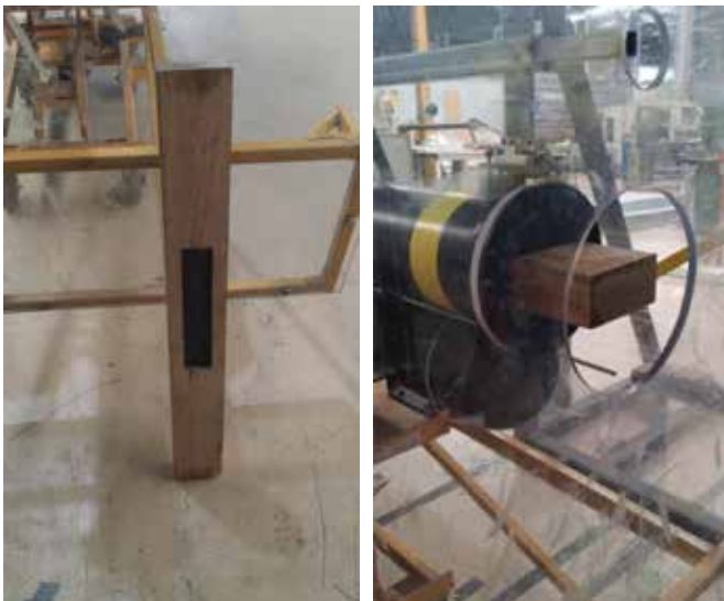
Figure 5.8. IMOC Windborne Debris Testing Procedure. AZ/NZS 1170.2 specifies a 100-by-50-mm, 4-kg timber missile for Part 1 of the test, but does not specify a required length. Hence the testing facility generally takes a one-meter length, and fits steel blocks to the inside to achieve the required mass (left). Note that during the firing, witnesses stand behind a transparent safety barrier a few meters away (right). © JML-Craft
