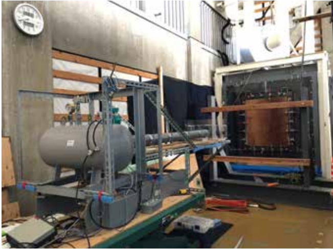
Figure 7.4. Air cannon for missile impact-testing of glazing, DPRI, Kyoto University. © Angela Mejorin
