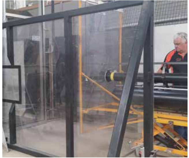
Figure 5.7. IMOC Windborne Debris Testing Procedure. The air cannon is placed 2 meters away from the testing specimen and the nozzle is approximately 1.2 meters from the ground. The cannon is only able to achieve velocities to the nearest whole number, as read on a gauge. Once the desired velocity is reached, the missile is released from the cannon. © JML-Craft
