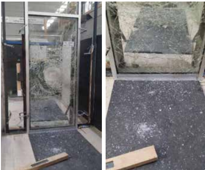
Figure 5.12. IMOC Windborne Debris Testing Procedure. The glass panel impacted by 4-kg timber missile at 40 m/s. Both lites of the outer pane shattered, however the PVB was not penetrated, and the timber missile landed in front of the panel. The back pane shattered. The edges of the imprint were deeper than the center. The missile front surface was flat. © JML-Craft
