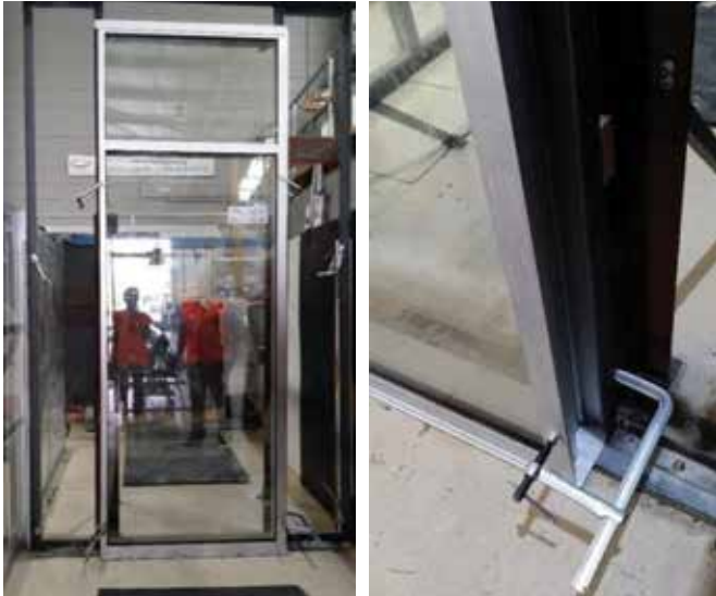
Figure 5.6. IMOC Windborne Debris Testing Procedure. (Left) The testing specimen should arrive at the laboratory as it would be delivered on site. This will account for effects due to the degree of rigidity between the glass and its frame. (Right) For four-sided fully-framed glass, the frame was clamped to vertical posts on either side of the mullion. © JML-Craft
