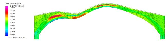
Fig. 9 Deformed shape and Mohr-Coulomb stresses for the actually built bridge with a force equal to 1,000 (kN).
