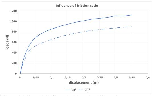
Fig. 15 Pushover analysis of actually built bridges having different values of friction angle.
