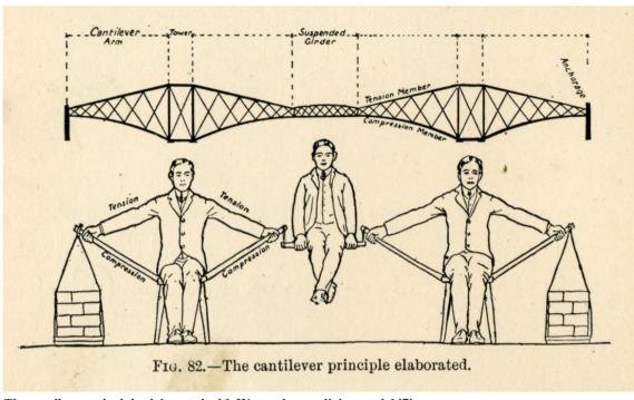
Fig. 3 The cantilever principle elaborated with Watanabe as a living model [7].
