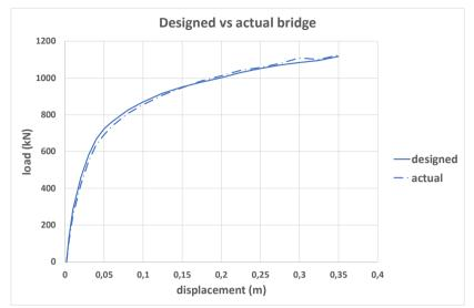
Fig. 10 Pushover analysis of designed and actually built bridges having masonry with c = 1.0 (MPa) and fill with c = 0.2 (MPa).
