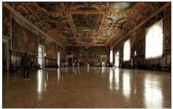
Fig. 5 Largest room of the Doge's Palace, called "Sala del Maggior Consiglio" (53.8 m long, 26.2 m wide, and 15.5 high), whose ceiling and roof are supported by larch lattice trusses and purlins. Each timber tie-beam consists of four pieces joined by "Jupiter dart" connections. On the mainland, those rooms were often roofed by masonry vaults.
