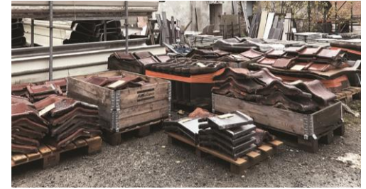
Fig. 2 – Rotor DC storage area for building components salvaged from deconstruction sites, later prepared for reuse and sold, Brussels, December 2019. Credits: the authors.
