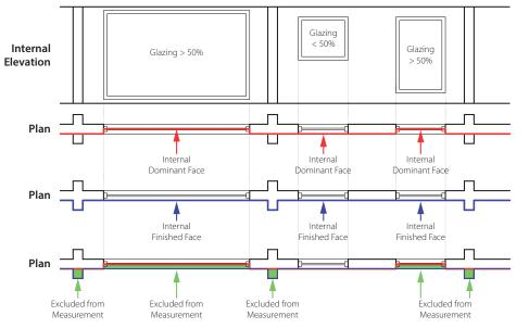
Figure 6. Comparison of Internal Dominant Face (used in IPMS-2 definition) with Internal Finished Face (to be used in defining the new IPMS-4 definition).
