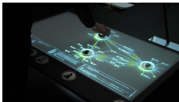
Fig. 5: The user moves the fiducial markers on the digital interactive table to visualize the people's networks (Source: ImpulsBauhaus in 3 minutes, https://vimeo.com/5333614 )
