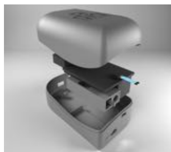
Fig. 7.2 - Render components and how they were placed inside
