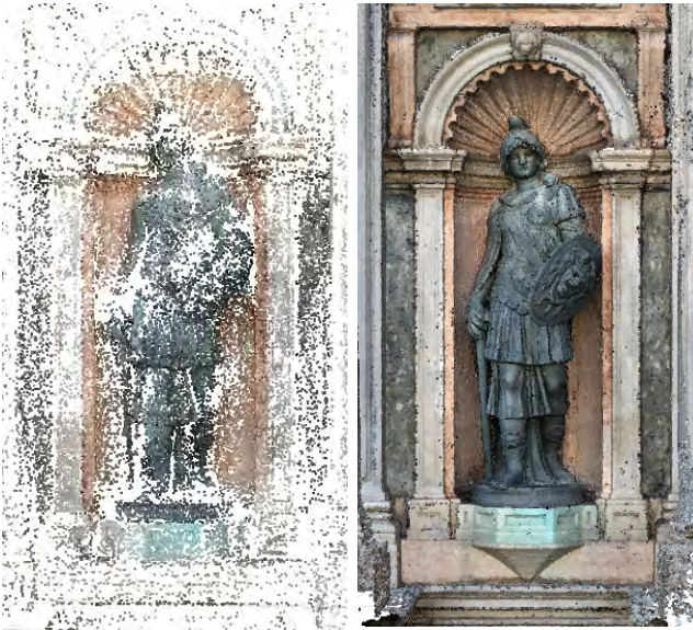
Figure 17. Tie points and dense cloud of the photogrammetric model of Pallas.
