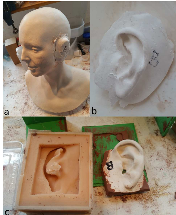
Figure 2. The making of a negative ear mold: (a) 1st negative mold; (b) Jesmonite® replica; (c) 2nd negative mold.
