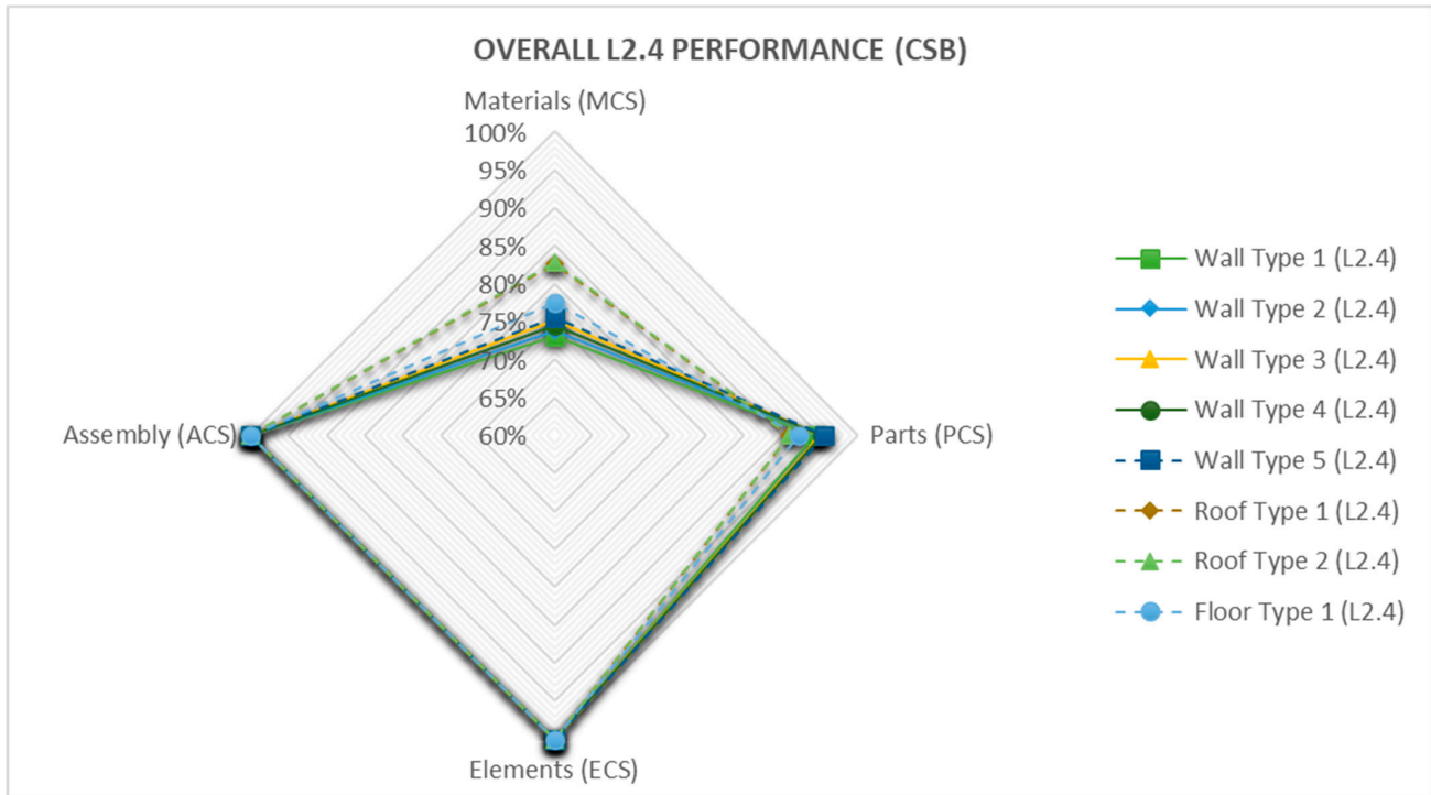
Figure 21. Overall circularity performance according to Level(s) indicator L2.4 (CSB).
