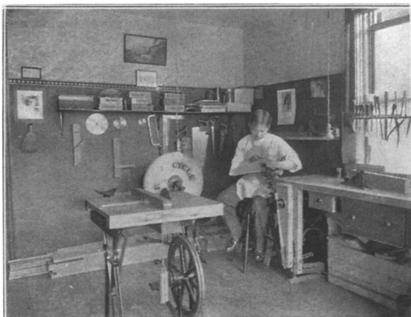
A Corner in the Author's Home Workshop, Showing the Bench, Circular Saw and Bicycle Grindstone
