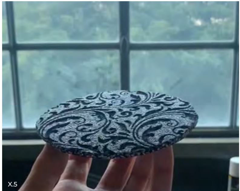
FIGURE X.5 - A study of surface decorations made by digital fabrication on recycled material from the soles of sports shoes. The aesthetics of the material change depending on exposure: when exposed to direct light, the workings on the material are barely perceptible, while against the light the texture becomes evident. Research commissioned by ESO, 2021 (Source: Chigos)
