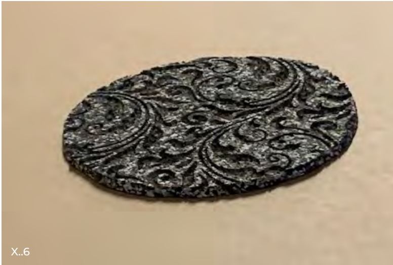
FIGURE X.6 and X.7 - A study of engraved (left) and cut (right) surface patterns on recycled materials from the soles of sports shoes. At low laser power values, it is possible to engrave the material without burning it; at higher power values, the laser burns the material and the texture becomes more perceptible even in situations of direct light exposure. Research commissioned by ESO, 2021 (Source: Ghigos)
