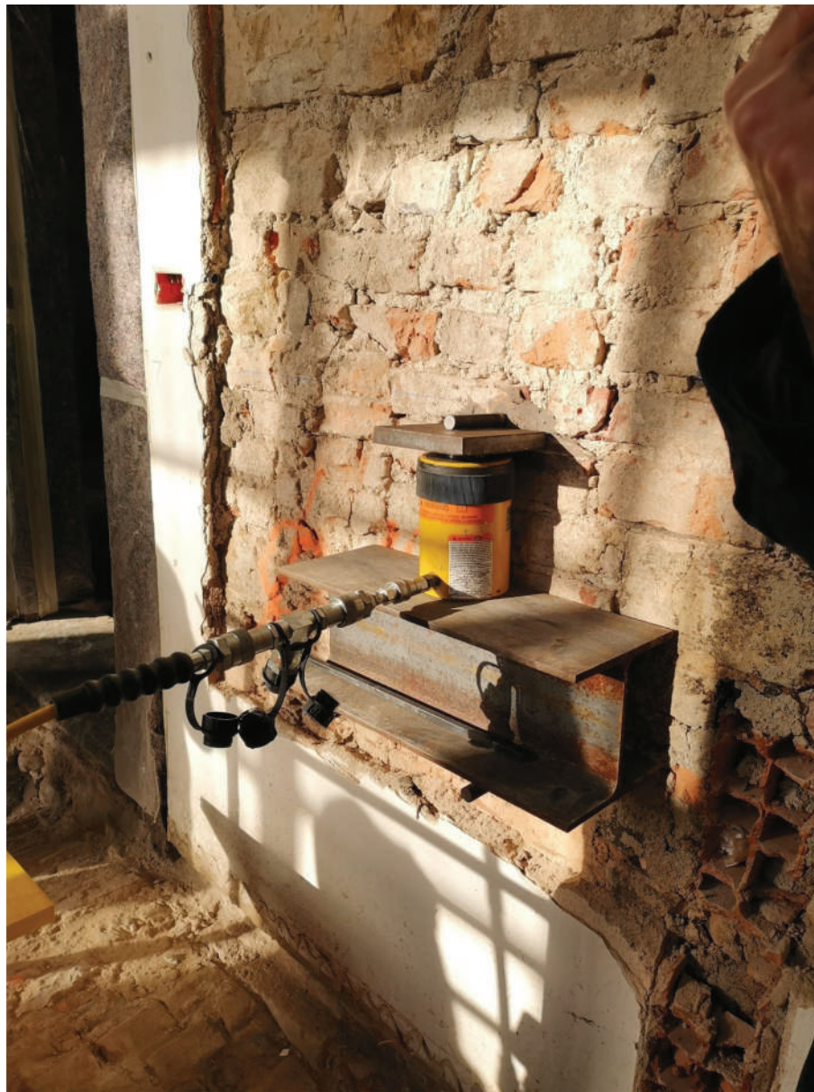
Fig. 6. Shear test performed using the procedure conceived and developed in this research activity. The masonry was made of bricks and lime mortar. Before executing this test, the plaster had been removed from the masonry. This test used the steel plate in lieu of the square-section steel bar.
