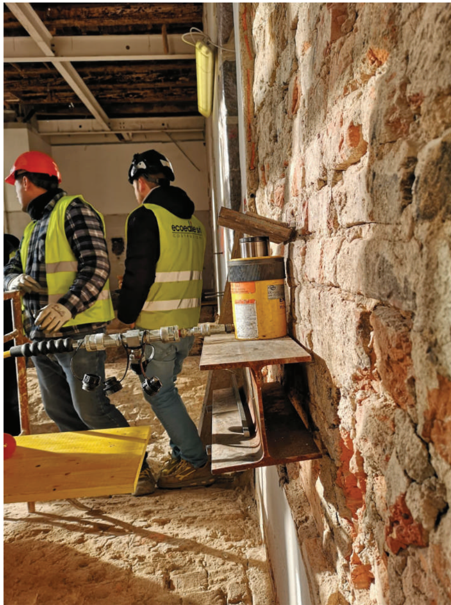
Fig. 9. Photo taken when the anchor had just collapsed. The image shows the test set-up and the tested anchor, which is bent upward. In all the tests the anchor reached rotations substantially larger than that induced by the peak of the force, with no more than moderate decrease in the force applied by the jack (pseudo-plastic post-peak behavior).
