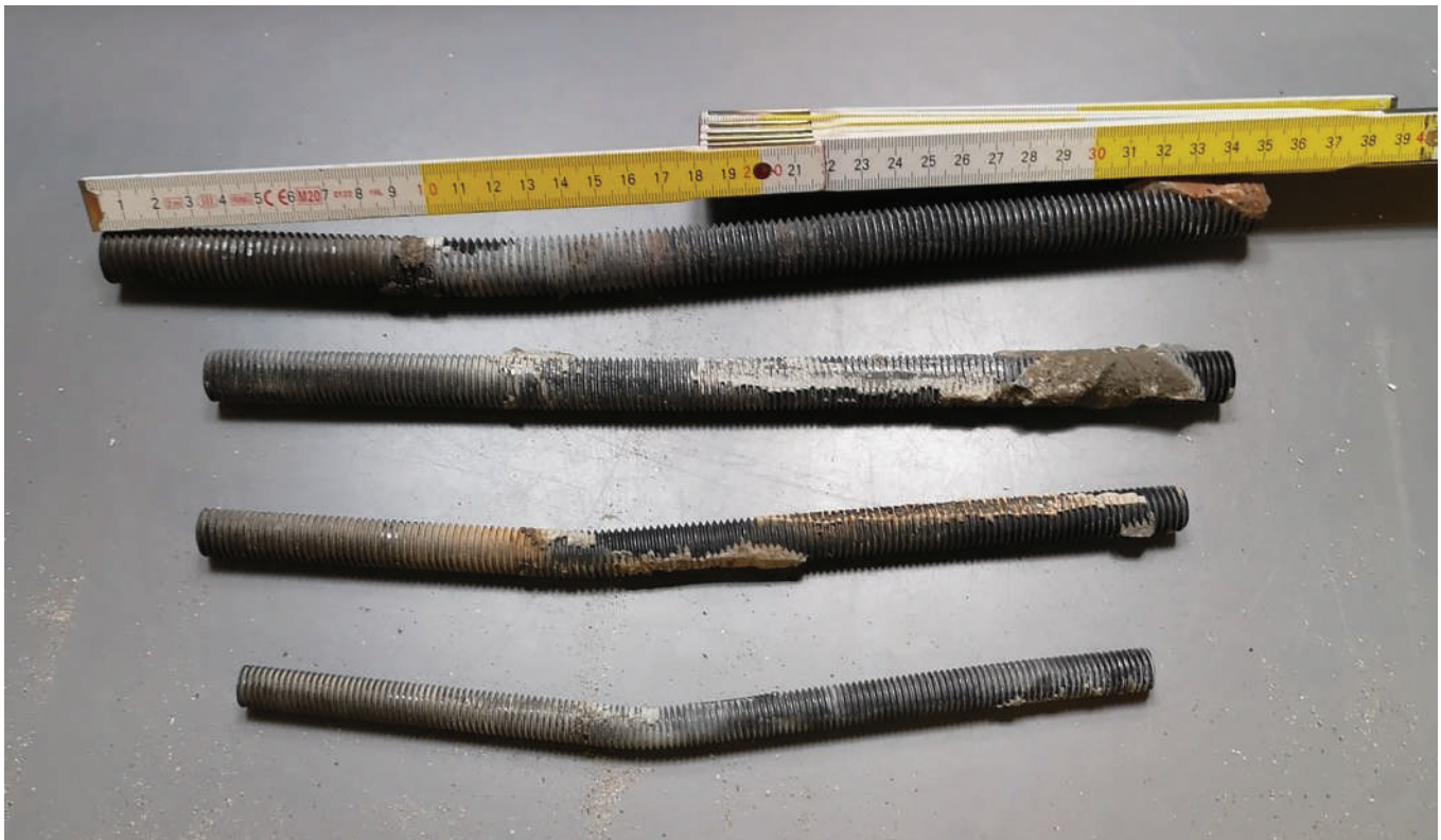
Fig. 14. Four anchors of different diameters and lengths, extracted from the masonry after the tests. All the anchors extracted from the masonry after the tests did not exhibit any plasticity in the embedded part (while the sections that emerged from the masonry surface exhibited large residual bending).
