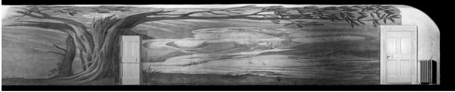
Fig. 11 Orthophoto of the wall surface of the western gallery on the first floor of the Convent of Trinità dei Monti. Digital elaboration of the point cloud showing the reflectance value in grayscale. Rendering by Cristian Boscaro/Imago rerum/Iuav
