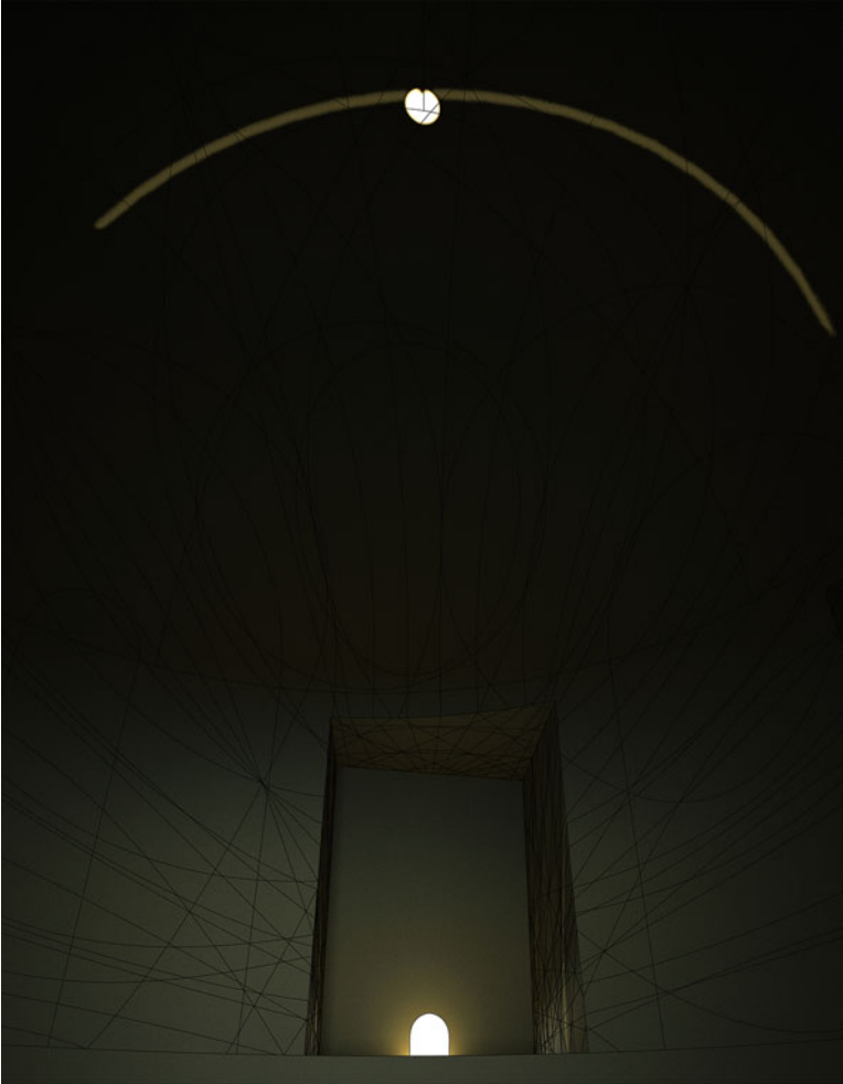
Fig. 38 Inner perspective view of the catoptric solar clock and projection on the vault of the light arc described in E. Maignan’s scientific reminder (point 6)
