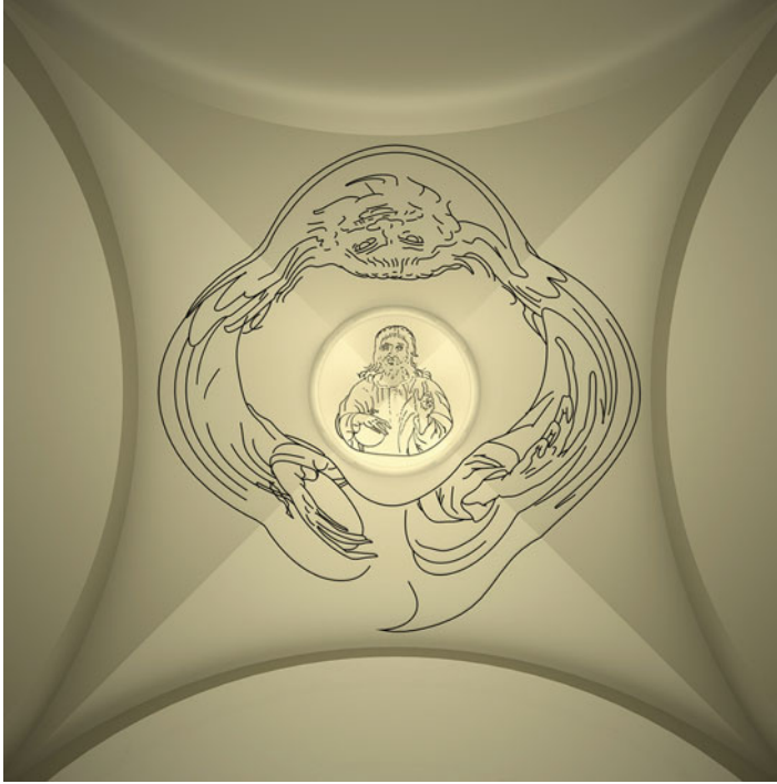
Fig. 16 Perspective view of Christ distorted image from the correct point view which is recognizable as a reflection on the conical mirror positioned on cross vault
