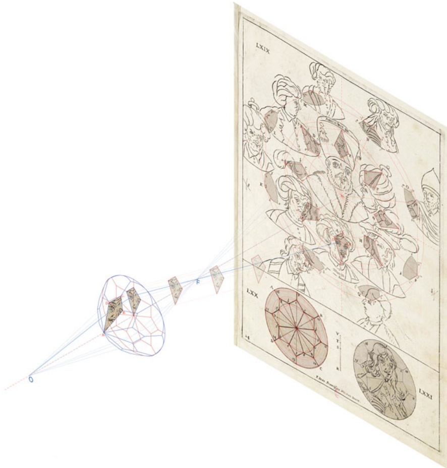
Fig. 23 The functioning scheme of Nicéron's game. The refracted portion of painting appears to be detached from the canvas surface (axonometric view)
